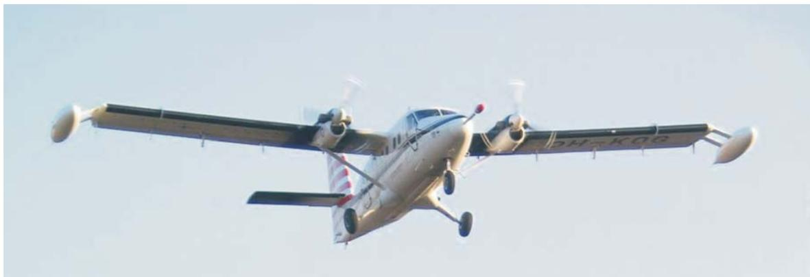
Fig. 1. Twin Otter aircraft with three-in-one aerogeophysical system
