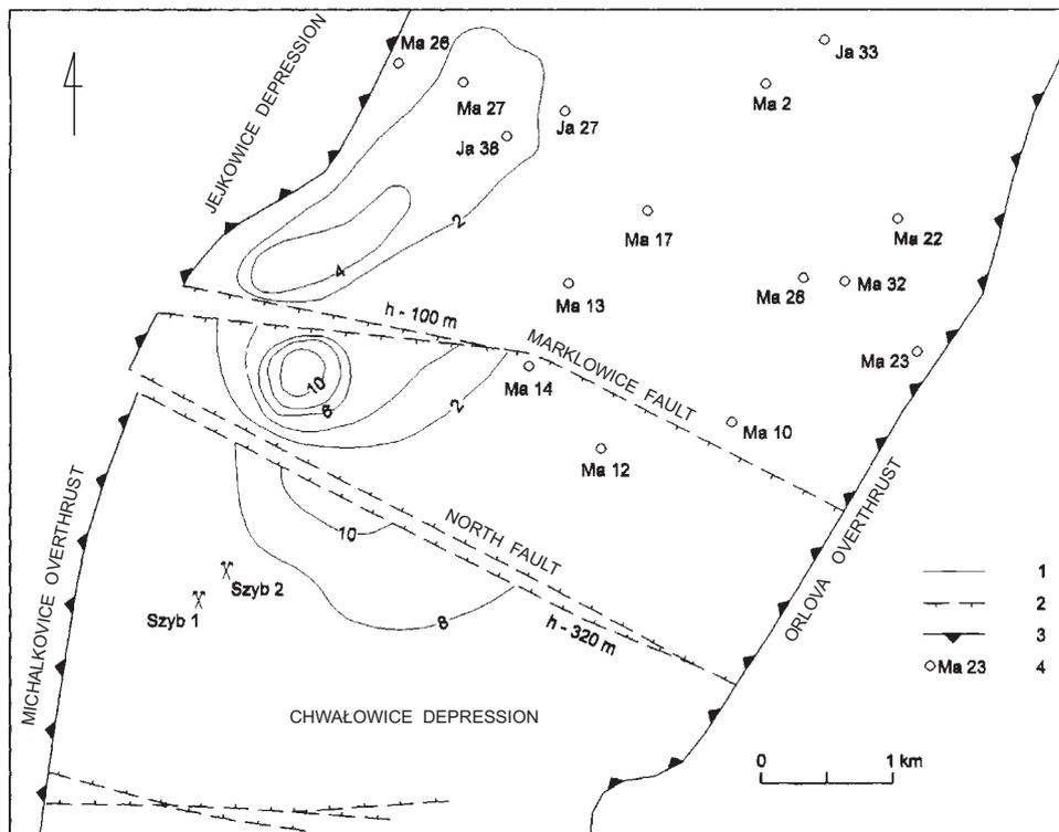
Fig. 3. Changeability of methane bearing capacity in the area of Chwałowice depression (level -580 m over sea level)
