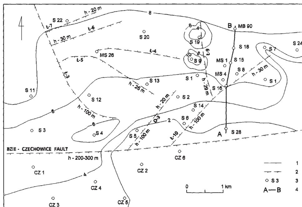
Fig. 1. Changeability of methane bearing capacity in area of Bzie-Czechowice fault (level -800 m over sea level) (after Kędzior, 2000)
