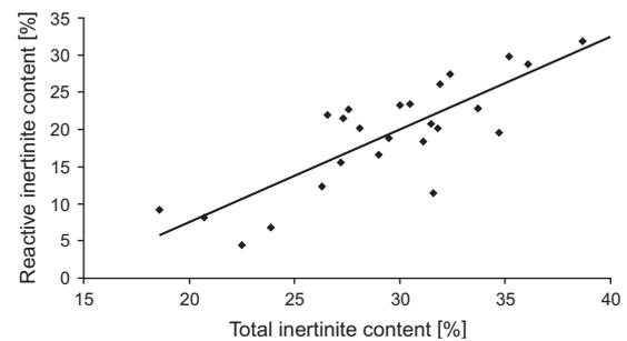
Fig. 4. Relation between total inertinite and reactive inertinite contents in feed coals from K-7 boiler. Correlation coefficient is 0.84
