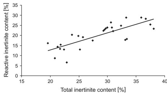
Fig. 3. Relation between total inertinite and reactive inertinite contents in feed coals from K-6 boiler. Correlation coefficient is 0.79
