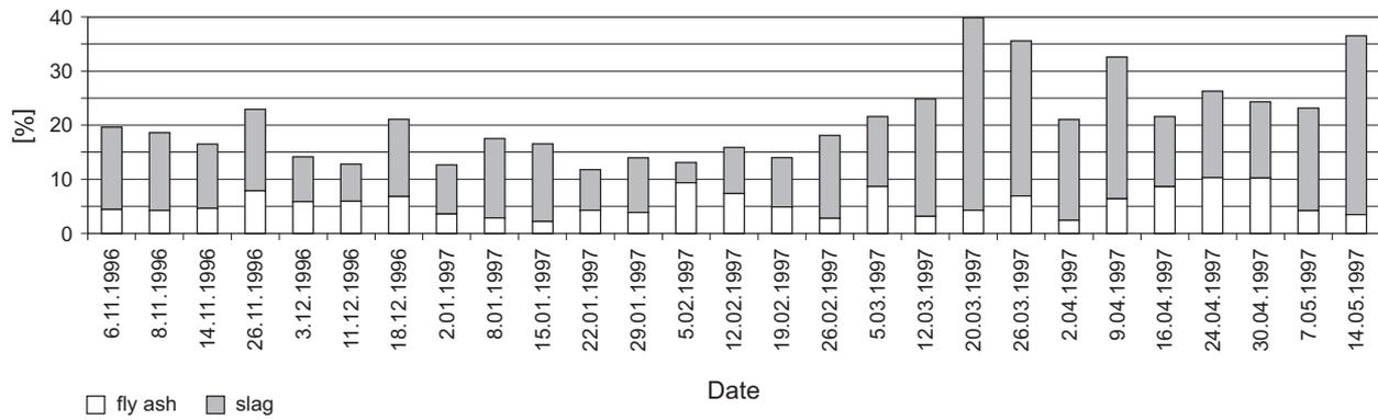
Fig. 1. Unburned organic matter content in slag and fly ash from K-6 boiler
