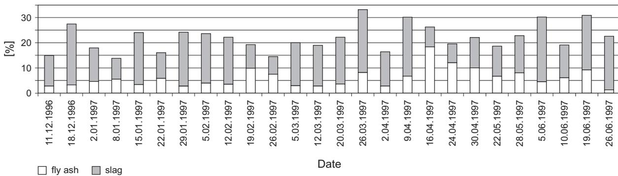
Fig. 2. Unburned organic matter content in slag and fly ash from K-7 boiler
