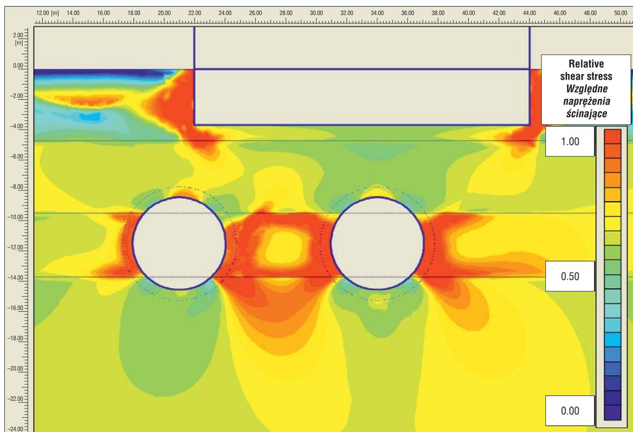
**Fig. 9.** Relative shear stresses (normalized by maximum stress) in construction zone in the cross-section plane to the metro line
