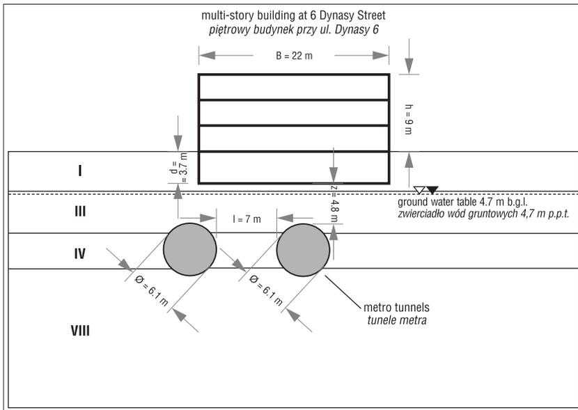
**Fig. 4.** Geometry of the tunnels project with soil layers numbered
