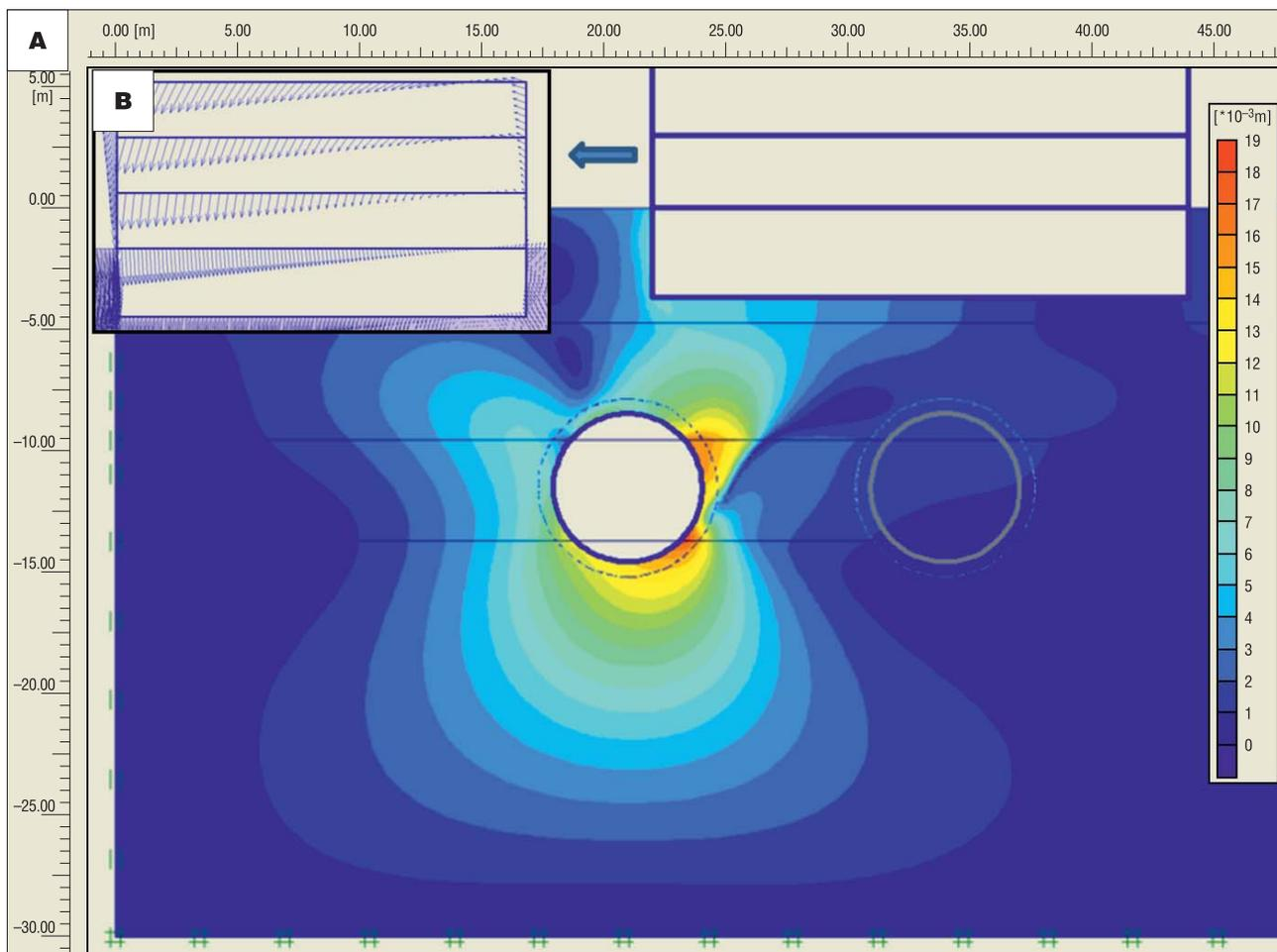
**Fig. 12.** **A** – total soil displacements induced by the southern metro tunnel; **B** – displacement vectors of the building at 6 Dynasy Street
