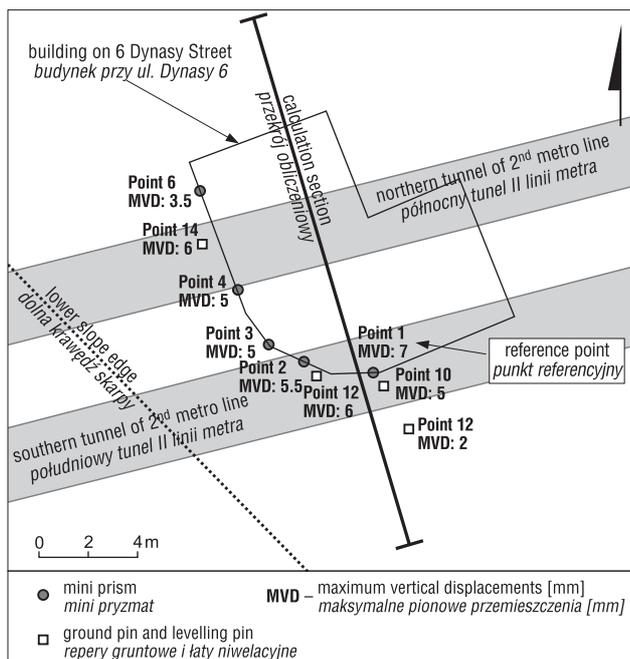
**Fig. 6.** Survey monitoring of a building at 6 Dynasy Street
