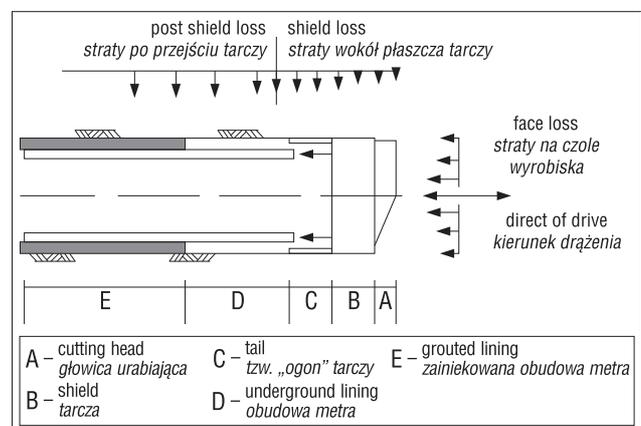
**Fig. 3.** Sources of volume loss in the TBM method (Potts & Zdravković, 2001)
