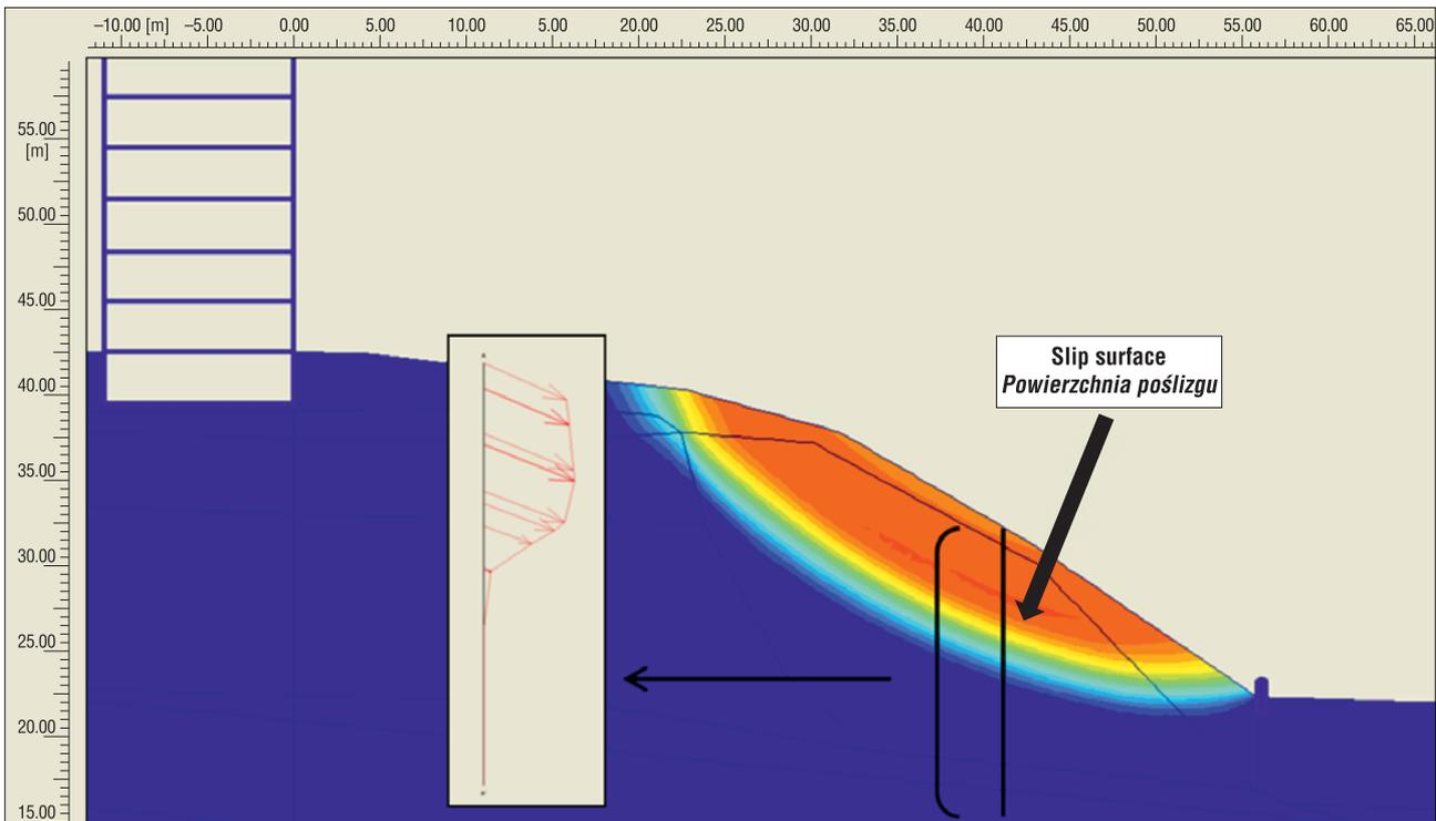
**Fig. 15.** The visualization of potential slip surface with a section showing vectors of displacement
