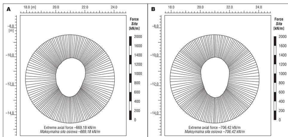
**Fig. 10.** Axial forces acting on: **A** – southern tunnel; **B** – northern tunnel
