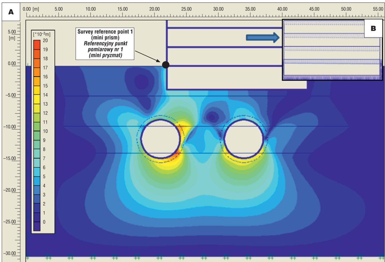
**Fig. 13. A** – total soil displacements induced by the two metro tunnels; **B** – displacement vectors of the building at 6 Dynasy Street
