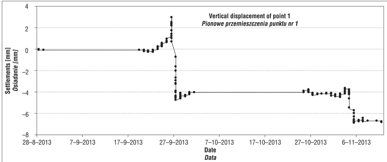
Fig. 7. Settlements of point 1 (mini prism) located on the building at 6 Dynasy Street against time (ZTM Warszawa, 2015)
