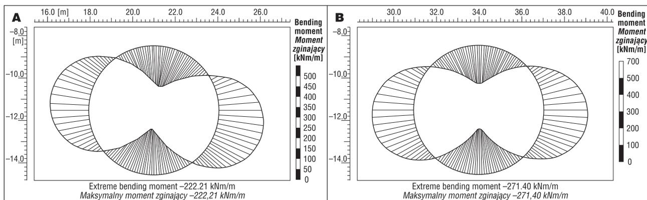
**Fig. 11.** Bending moments for metro construction below building: **A** – southern tunnel; **B** – northern tunnel
