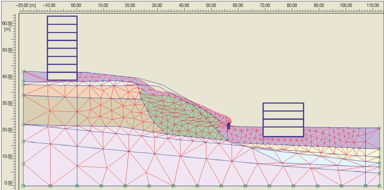
**Fig. 14.** Deformed mesh model affected by potential landslide
