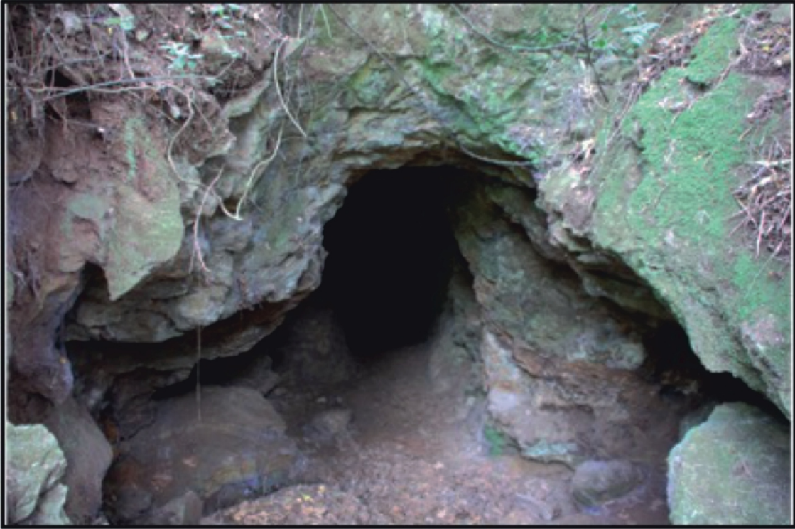
Fig. 16. Stope with a pillar near adit entrance, Maitland prospect Note the green secondary copper staining, produced by malachite or other copper minerals (from McLelland, 2018)
