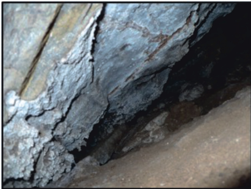
Fig. 17. Narrow dipping stope in the Maitland prospect The hanging-wall appears to be lined with secondary efflorescences, possibly sulphates derived from the oxidation of sulphides (from McLelland, 2018), or aragonite
