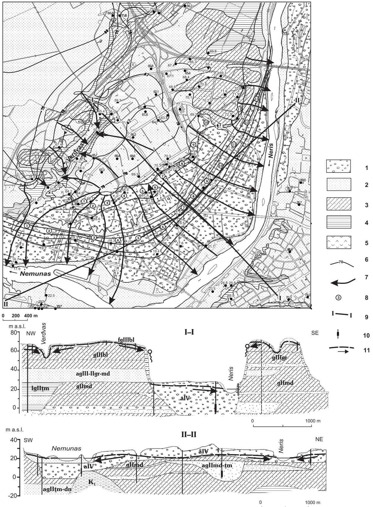
**Fig. 1. Hydrodynamic scheme of shallow groundwater outflow estimation in contact of alluvium and fluvioglacial sediments**
