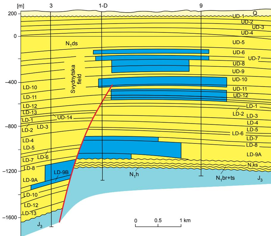
Fig. 2. Cross-section I-I of the Vizhomlia gas deposit
