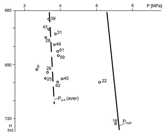
Fig. 5. Barosmotic head pressure ( $P_{o,h}$ ) in waters of the Svydnytsia gas deposit in UD-11 horizon
