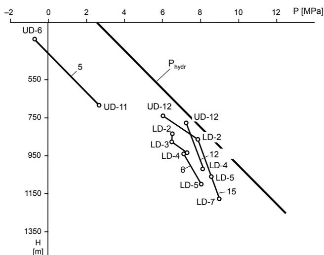
Fig. 4. Barosmotic head pressure ( $P_{o,h}$ ) in waters of the Svydnytsia gas deposit in boreholes
