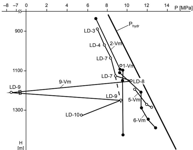
**Fig. 6.** Changes of barosmotic head pressure ( $P_{o,h}$ ) of water in boreholes of the Vizhomlia gas deposit
