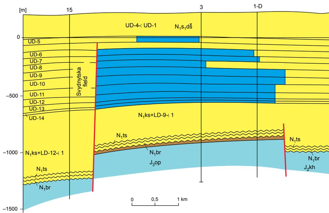
Fig. 3. Cross-section II-II of the Kokhanivka gas deposit
