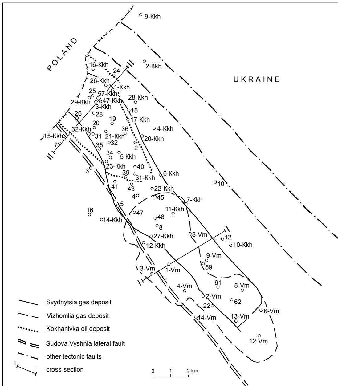
**Fig. 1. Outlines of oil and gas deposits and location of the most important boreholes in the Kokhanivka–Svydnytsia area**
