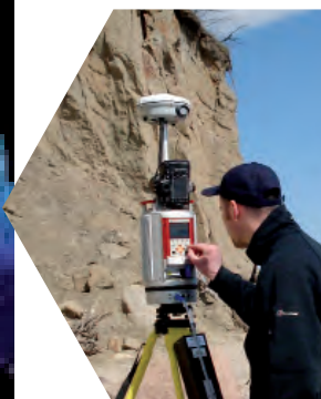
Scenes from a laser scanning – 3D model of the cliff in Gdynia-Orłowo
