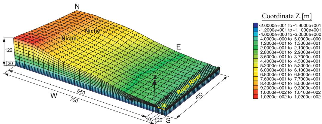
**Fig. 2. Spatial model of the Kawiory landslide slope**
