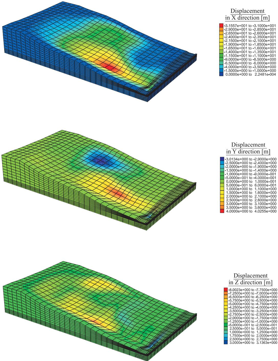
Fig. 4. Fields of displacement components in equilibrium state
