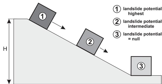
Fig. 6. Explanation of the “landslide potential” term
