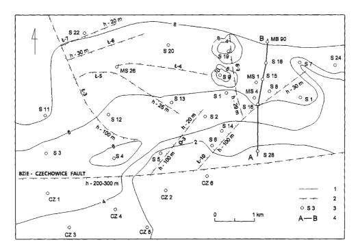
Fig. 1. Changeability of methane bearing capacity in area of Bzie–Czechowice fault (level –800 m over sea level) (after Kędzior, 2000) 1 — methane bearing capacity isolines, 2 — faults, 3 — surface boreholes, 4 — line of cross-section A–B
