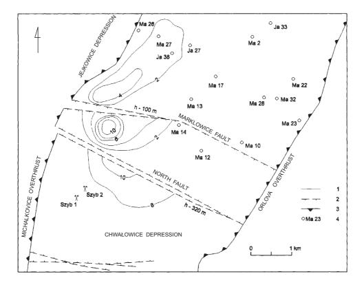
Fig. 3. Changeability of methane bearing capacity in the area of Chwałowice depression (level -580 m over sea level) *l* — methane bearing capacity isolines, *2* — faults, *3* — overthrusts, *4* — surface boreholes
