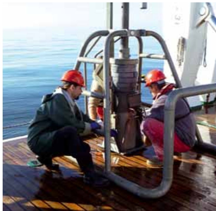
Getting a core out from a box-corer for lithological and chemical studies
