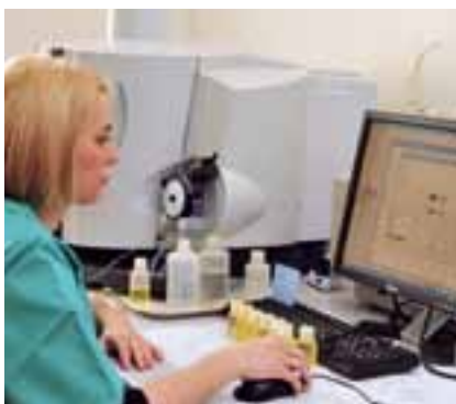
ICP – OES (inductively coupled plasma optical emission spectrometry (ICP-OES), and CAP 6500 DUO, Thermo-Scientific
