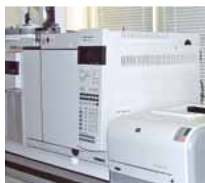
Gas chromatograph with detector and dual mass spectrometer GC-MS/MS, 7890A-7000A Agilent Technologies (USA)
