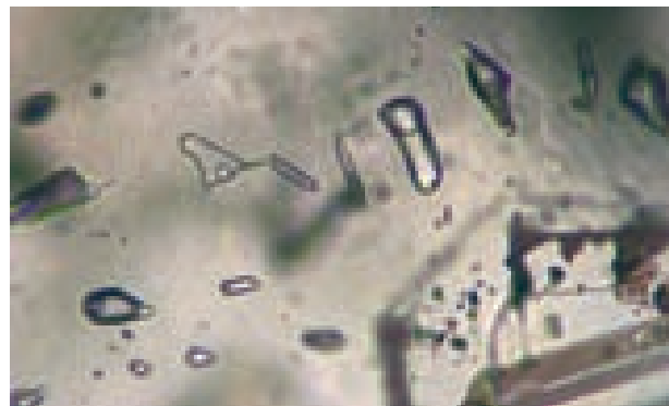
Generation of phases in the course of cooling of single-phase fluid inclusions
