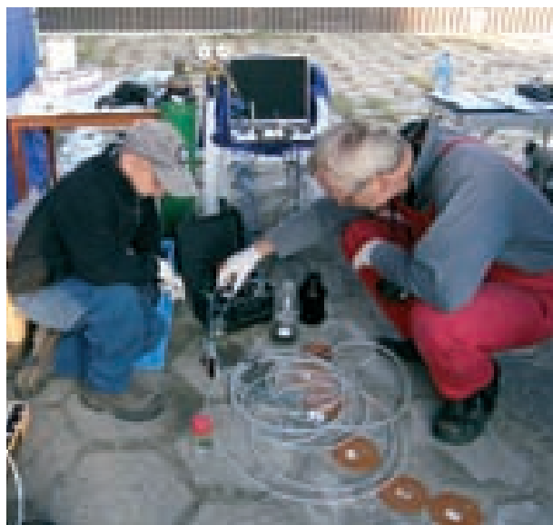
Taking samples from piezometer of the CMT type for photometer testing
