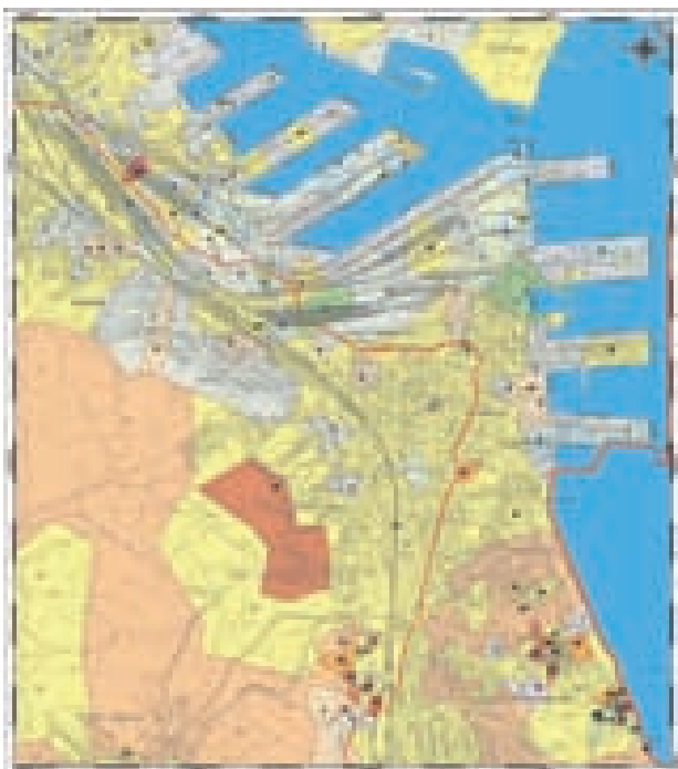
Map of soils occurring at the depth of 4 m below terrain surface (Engineering-Geological Atlas of the Gdańsk-Sopot-Gdynia in the scale 1:10,000)
