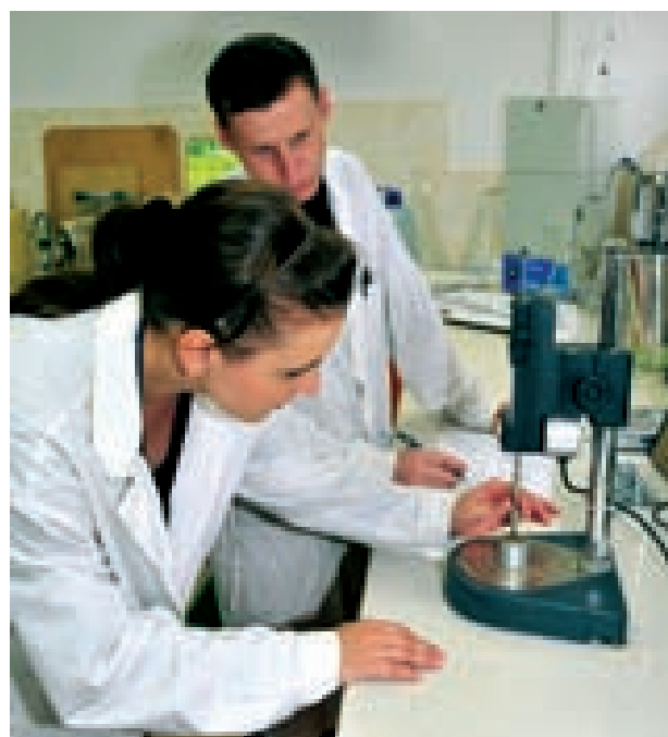
Liquid limit determination of soil using drop-cone penetrometer
