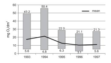
Fig. 2. Extreme and average BOD<sub>5</sub> values of water samples from the Cicha Woda stream at the Zakopane-Harenda measuring point
