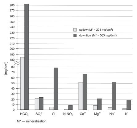
Fig. 4. Water chemistry changes in the Orawców stream around the municipal waste landfill
