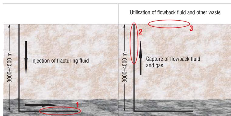
**Fig. 6.** A scheme of theoretical routes of pollutants migration (1 – from the horizontal section of well, 2 – from the near-well zone of its vertical section, 3 – from the surface)
