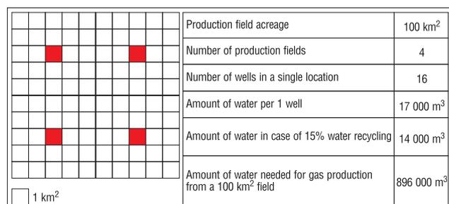
**Fig. 4.** Schematic development of an area of 100 km<sup>2</sup> and an estimate of the amount of water needed for shale gas production in this area
