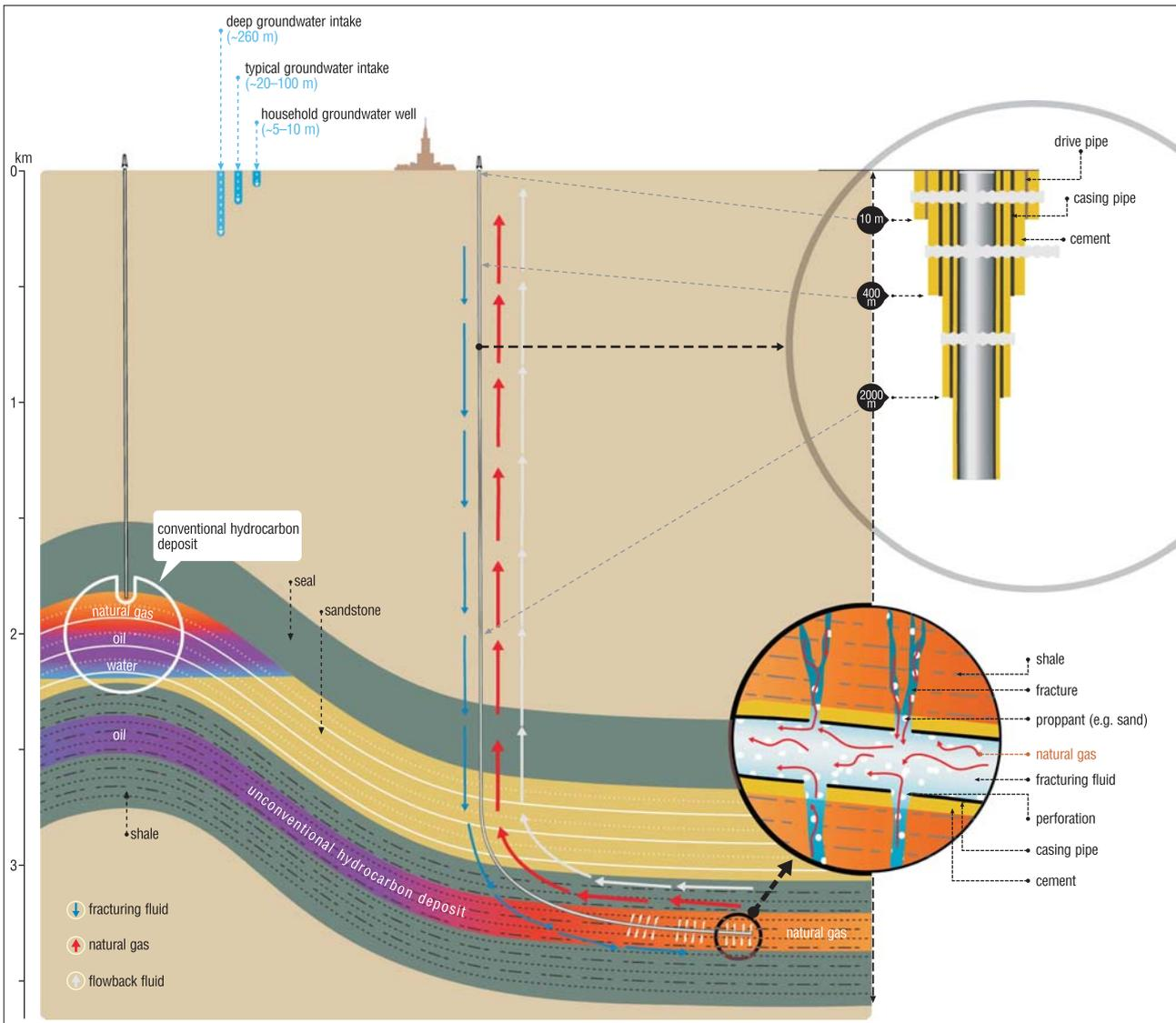
Fig. 3. A scheme of hydraulic fracturing process
