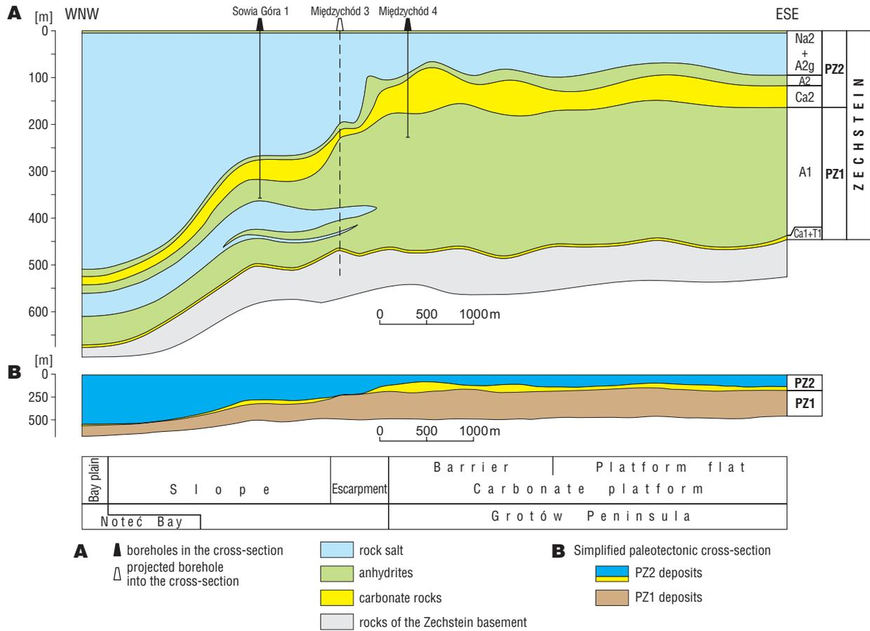
**Fig. 2.** Paleotectonic cross-section at the top of the PZ2 cyclothem based on the A1 Międzychód–Sieraków 3D seismic section. Seismic section after Górska and Łukaszewski (2003)
